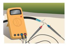
Regularly measure Ohm resistance and insulation resistance, minimum: before, during and after installation.
