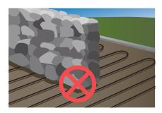
Do not install heating elements under walls and fixed obstacles. Min. 6 cm space is required. Keep elements clear of insulation material, other heating sources and expansion joints.
