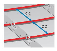
**Note!** Heating cable bending diameter must be at least 6 times cable diameter.
