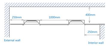
Note. When recessing into a T-tail grid ceiling, a proprietory accessory bridging bracket required.
