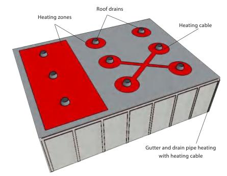
protection of flat roof areas (4). This is the most effective way to protect the roof against snow, however it requires larger installation in terms of of heating output than any described above.
