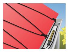
6. Install DEVIreg<sup>™</sup> 850 external sensor, if any, in the gutter according to the sensor manual.
