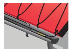
Extend sensor cables, cold tails/terminate cables and place connections dry. Seal all penetrations, e.g. through roofs and walls.
