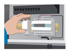
Check once again and compare the insulation resistance and Ohm rating for cables. Install DEVIreg<sup>™</sup> thermostat and connect cables to the connection boxes and to the switchboard.
