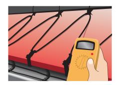
Install the cable(s) on the roof, in gutters and downpipes. Check once again and compare the insulation resistance and Ohm rating for constant wattage cables.
