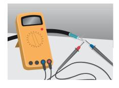
3. Check the insulation resistance and also Ohm rating for constant wattage cables. Install the cable(s) on the roof, in gutters and downpipes.
