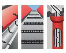
Install the connection box and fixing accessories in the gutters, gutter valleys, on the roof and/or the cable.
