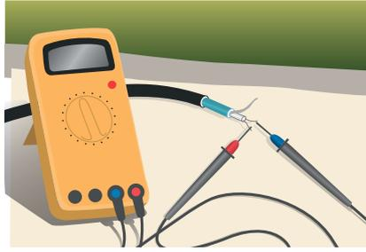
Regularly measure Ohm resistance and insulation resistance, minimum: before, during and after installation.
