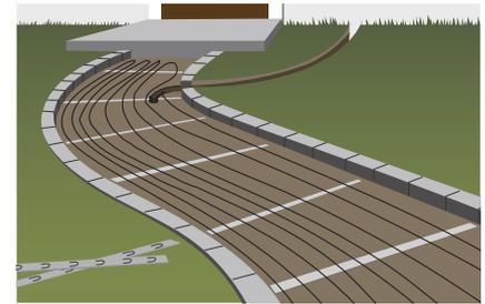
Prepare installation surface with DEVIflex™ fastening accessories and/or mesh reinforcement.
