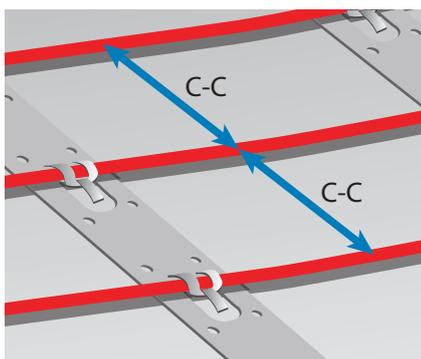
**Note!** Heating cable bending diameter must be at least 6 times cable diameter.
