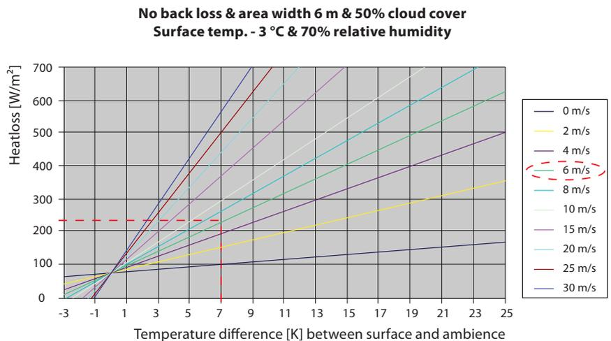
Fig. 3. Wind and temperature dependent heat loss
