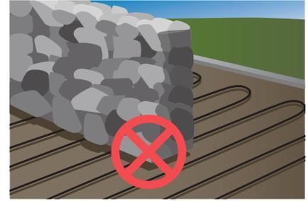
Do not install heating elements under walls and fixed obstacles. Min. 6 cm space is required. Keep elements clear of insulation material, other heating sources and expansion joints.
