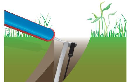
After laying blocks or pouring concrete/asphalt, install external sensor(s), and extend sensor cable(s) according to the sensor manual.
