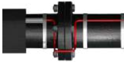
Example of cable mounting on a flange.
