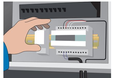
8. Check once again and compare the insulation resistance and Ohm rating for cables. Install DEVIreg™ thermostat and connect cables to the connection boxes and to the switchboard.
