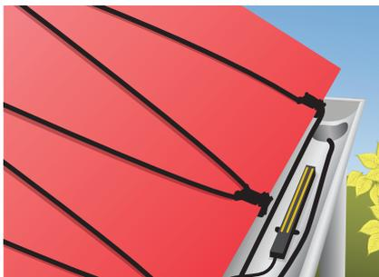
6. Install DEVIreg™ 850 external sensor, if any, in the gutter according to the sensor manual.
