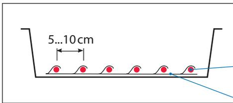
The DEVIfast™ is fixed by means of hotmelt, silicone, etc., but the best decision would be by screws or rivets.
