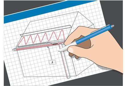
2. Develop the layout plan for cable(s), sensors and thermostats, cable connections/ cold tails, connection box, cable paths and a switchboard. Refer to DEVIreg™ 850 manual for location.
