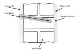
Installing the indoor sensor
