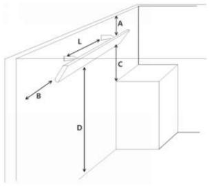
Note: When mounting single heater direct to a ceiling, there is a minimum clearance of 90mm (130mm recommended). For more details, see installation guide (available on request).
