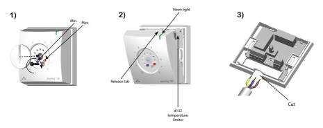
When installing a thermostat from Devireg<sup>™</sup> 130 Series, you must first remove the front cover.
