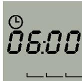
By pressing the ● the start time of the period starts blinking. You change it with the arrow buttons ▼▲ in increments of 15 minutes.
