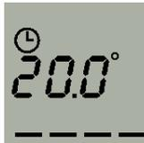
By pressing the ● the preset comfort temperature starts blinking, along with all the upper period bars ██████████ to symbolise the upper temperature.
