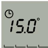
By pressing the ● the preset savings temperature starts blinking, along with all the lower period bars ██████████ to symbolise the lower temperature.
