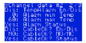
Data on the picture above means the following: **Temp Alarm** is disabled for **Channel #2 (Dis)** and Software does not control alarm temperature, alarm range set up with values from  $0 \,^{\circ}$ C to  $60 \,^{\circ}$ C, actual temperature of the sensor out of the range – **Alarm Status** = **Yes**.
